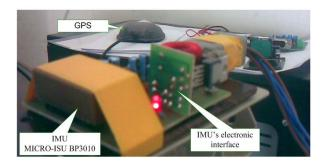
Fig. 1. IMU MICRO-ISU BP3010 and electronic circuits
