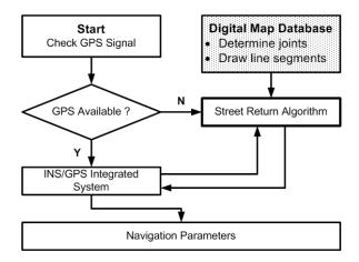
Fig. 3. Diagram of the proposed system
