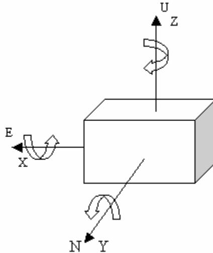
Figure 2: Initial IMU position for up-down calibration.
